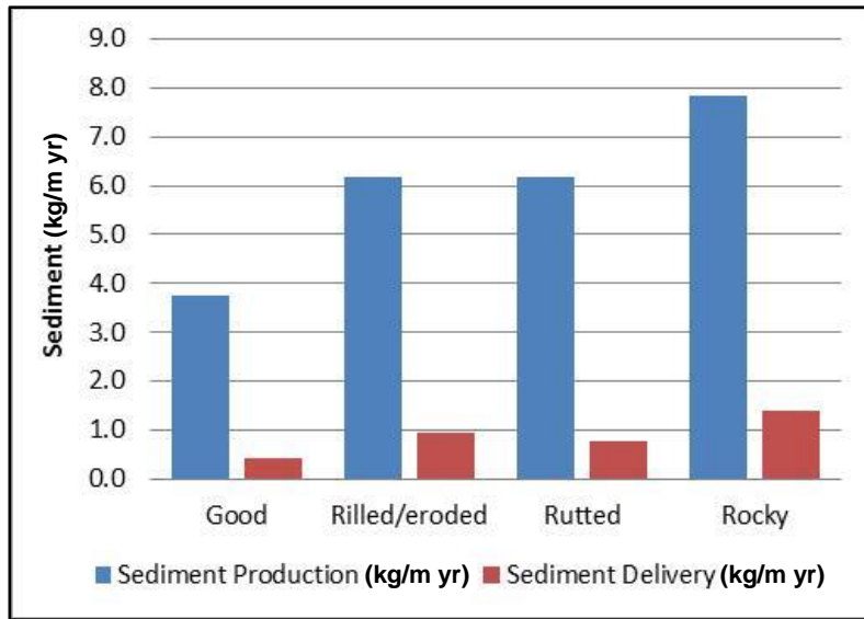
Figure 15. Normalized sediment production and delivery by road surface condition. The values are normalized by road length for each surface condition category.
